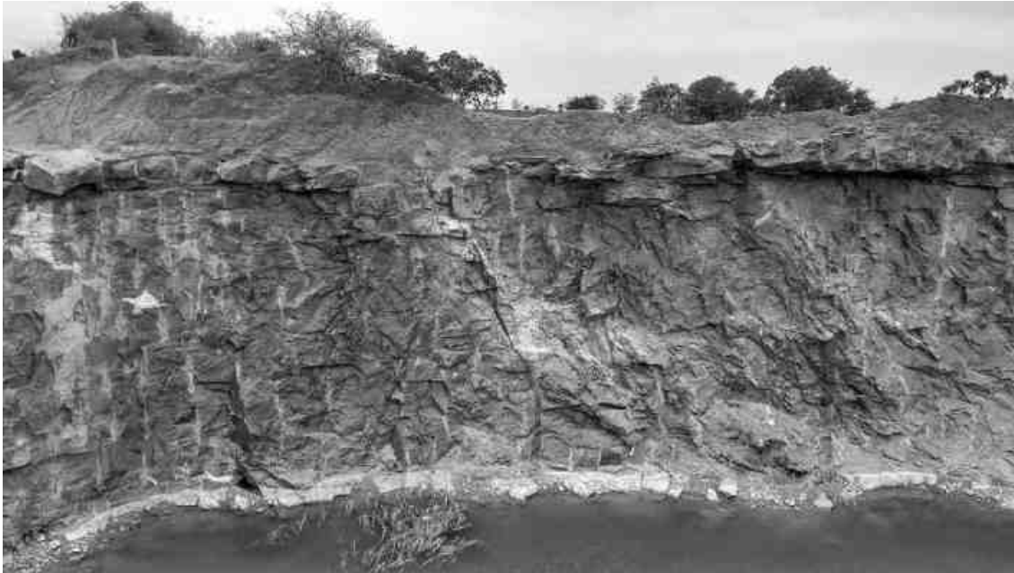
Aravakurchi, Thennilai East, Rough Stone Charnockite, E-W trending 60^{\circ} - 70^{\circ} northly dipping latitude 10^{\circ} 57' 57.20'' Longitude 77^{\circ} 52' 33.92'' .
