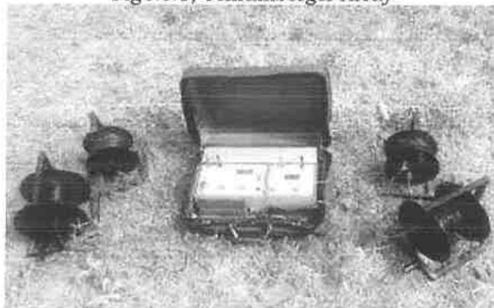
Fig No: 2. Model DDR-3 Electrical Resistivity Meter
